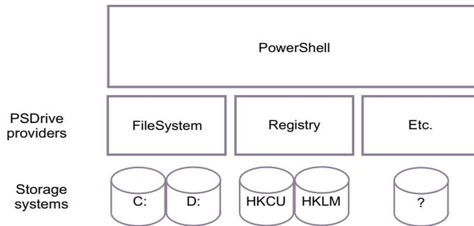
**Figure 2.2** PSDrive providers adapt different forms of storage so they look like disk drives within PowerShell
